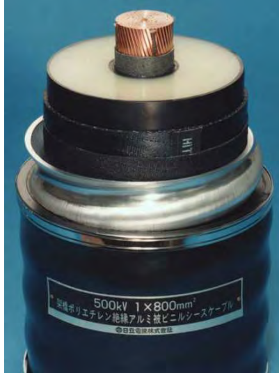
Figure 7.1(d): The World's First 500 kV XLPE Cable
