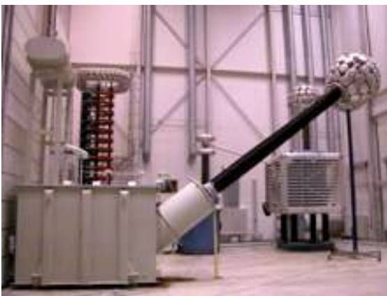
Fig 4. transformer prototype in the test laboratory
